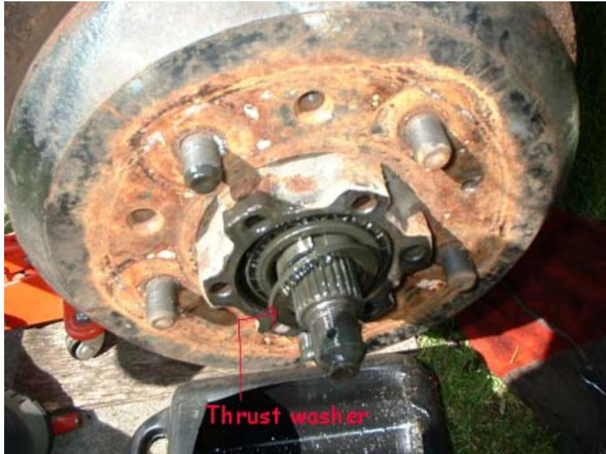
So now time to remove the hub and drum (if still fitted) and start to inspect the components.
