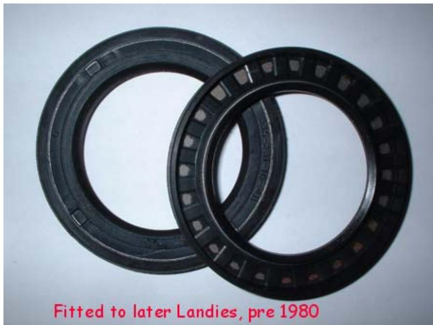
Now a look at the later type of seal, as fitted to axles made after 1980, again, the top seal is showing the inside (i.e. facing the inner bearing)
