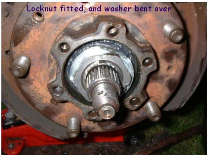
Then replace the drive flange and halfshaft. Use a new paper gasket between the hub and drive flange.
