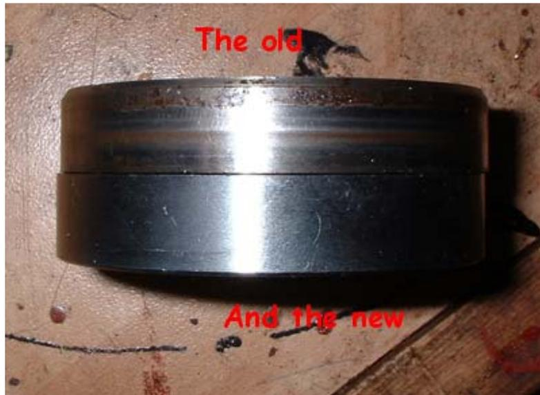
No need to remove the stub axle though (the one in the photo was removed as part of a full axle rebuild) as you can remove the land by first cutting into it a bit with a hacksaw, and then driving a sharp cold chisel into the slot you cut. This will split the land, and it will come off easily. Once it is off, it is a simple matter of pressing the new 'land' onto the stub axle...it is a tight interference fit.
