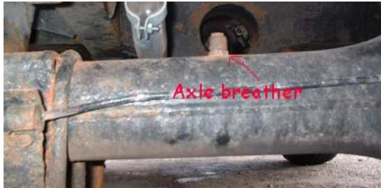
Remove the brass bell-shaped fitting on the top of the axle, and give it a shake. There is a ball bearing in there, which will rattle if the breather is not completely blocked with dirt, if it does rattle, try blowing through the breather, as sometimes the outer part can be blocked with dirt, even if the ball bearing rattles inside. It is possible to clean them out with a bit of wire and some petrol, or WD40, though. It just needs a bit of patience!
