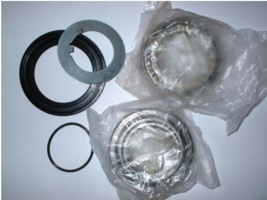
Back to business...Remove the hub oil seal by levering it out using a pry-bar, or a big screwdriver. Remove the inner bearing and clean all the components carefully. Inspect the bearings and race very carefully, any sign of scoring, or wear on the tracks; or any signs of grittiness when the bearings are run on the races, then the bearings must be replaced. If one is okay, and the other isn't, replace them both. Replacing just one is false economy.
