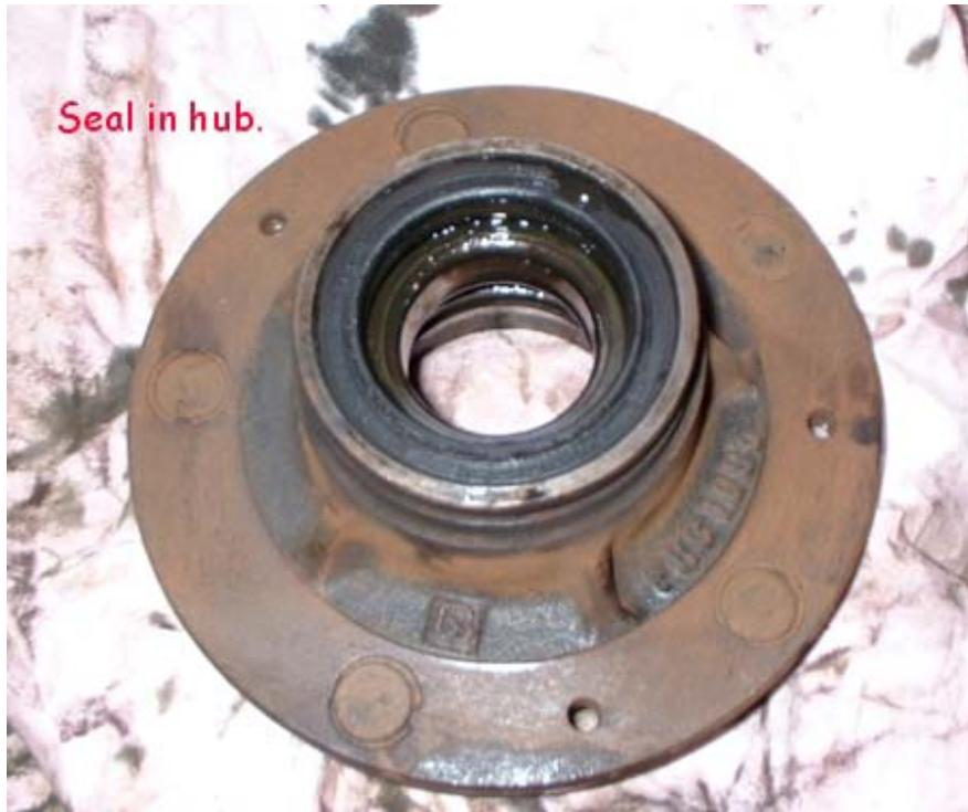
You might use a big socket or similar for this, but it is important that the seal goes in evenly, and the lips are not damaged. The later type of seal, with two lips, as fitted to 1980 onwards axles should fit so that the outer of the lips is about 1mm below the hub casing. It has a lip on the outer edge of the seal too, and this should end up flush with the hub casing.
