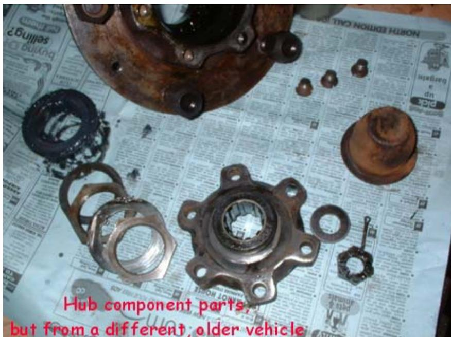
A quick look now at the new bits you will need. This next photo shows the original type of seal fitted to the hubs on early
