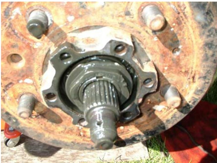
Now undo the three screws holding the brake drum in place, and pull off the drum. Don't forget to back off the brake adjusters first!
