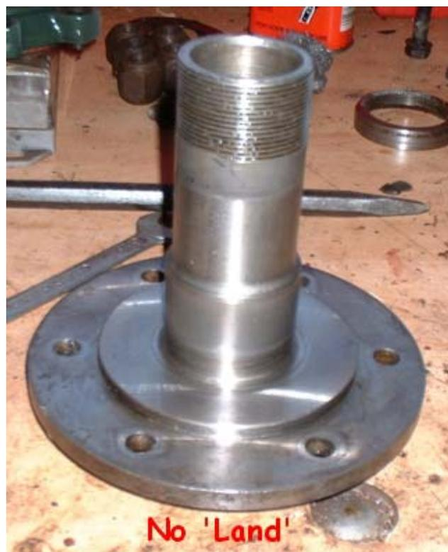
The above photo's show a stub axle from an earlier axle, before and after removing the 'land', if the land is scored or worn as in the next photo, it will need to be removed and replaced with a new one.
