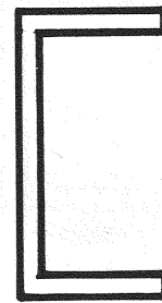
Cross-section of typical competitive vehicle chassis-member.
