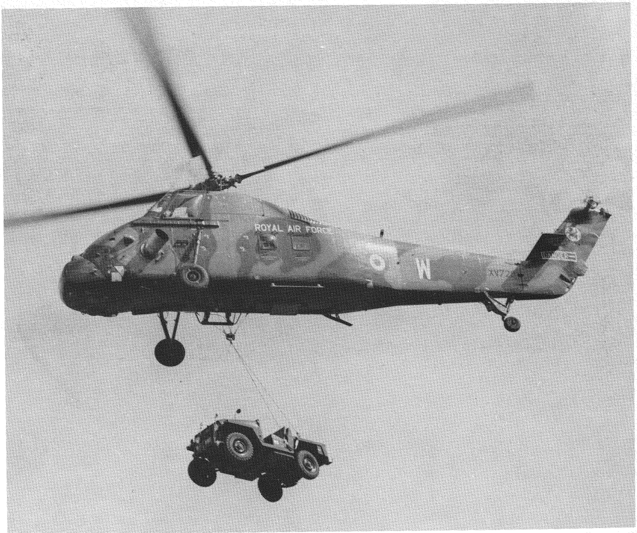
A Land-Rover 'half-tonne' being lifted by a Wessex helicopter of the British Royal Air Force
