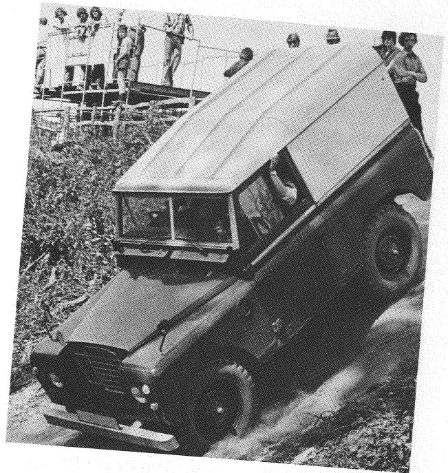
A Land-Rover can 'walk' down a steep slope quite safely by relying entirely on the engine to control the wheel speed
